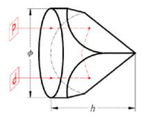
Corner Cube Prisms, which have three mutually perpendicular surfaces and a hypotenuse face, are designed to reflect any ray or beam entering the prism face, regardless of the orientation of the prism, back onto itself. A mirror will only do that at the normal angle of incidence. There are three total internal reflections within the corner cube.
